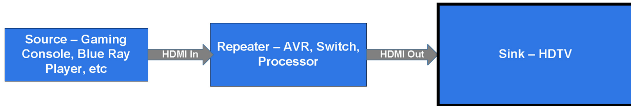
Connection Diagram Fresco SIX-G
